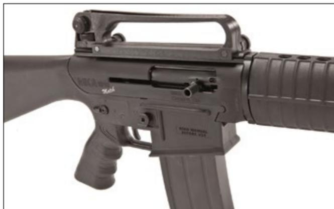
The MKA 1919 Match comes with an AR-style carry handle/rear sight that can be removed for adding sights and optics to the top rail. Also note the shotgun's enlarged, right-side-mounted charging handle.
